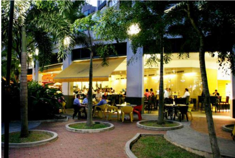
Figure 3-1: Awnings are to complement the scale and rhythm of the development façade, e.g. correspond to the column locations. Applicants should also seek clearances from SCDF on the location and extent of protrusion from the building façades.
